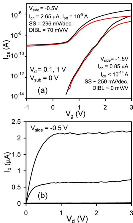
FIG. 2. (Color online) Electrical characteristics of an ultranarrow channel device. Estimated channel width is 7 nm. (a) Transfer characteristics for  $V_{\text{side}} = -0.5$  and  $-1.5$  V and  $V_d = 0.1$  V (red) and 1 V (black). Subthreshold behavior indicates charge trapping and detrapping events at the side silicon-silicon nitride interfaces. Drain induced barrier lowering (DIBL) is very small. (b) Output characteristics for  $V_{\text{sub}} = 0$  V and  $V_g = 0-3$  V and 1 V steps.
