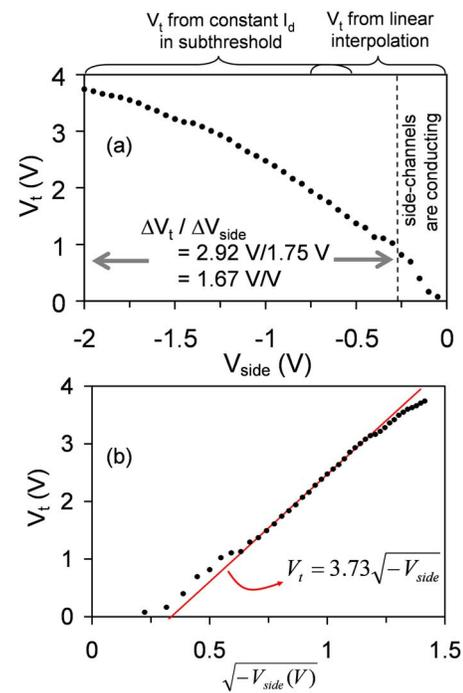
FIG. 3. (Color online) (a) Threshold voltage response to  $V_{\text{side}}$ , extracted using constant current method in subthreshold regime and linear interpolation in the “on” regime. (b)  $V_t$  graphed as a function of square root of  $-V_{\text{side}}$ .
