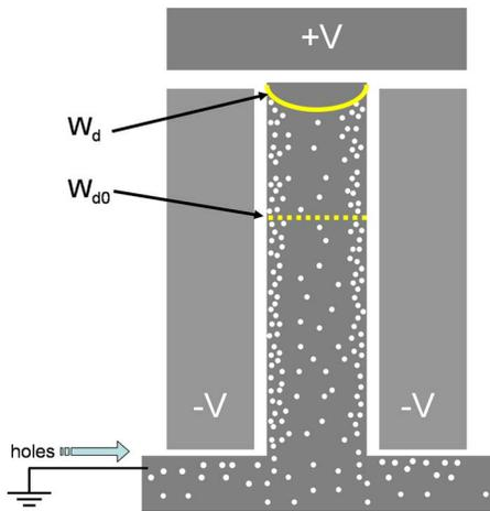
FIG. 4. (Color online) Cross-section schematic illustrating accumulated body operation. Holes are drawn from the substrate, connected to ground, into the device body.  $W_{d0}$  is the depletion depth under the top gate for a wide device. In the ultranarrow channel device  $W_{d0}$  is reduced to  $W_d$  due to accumulation of the body with holes when a large negative  $V_{side}$  is applied.
