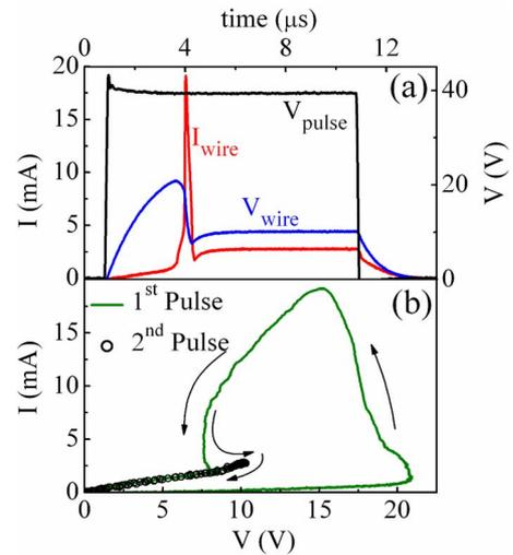
FIG. 4. (Color online) An *n*-type wire with  $L=4.0 \mu\text{m}$ ,  $W\sim 200 \text{ nm}$ , and thickness  $\sim 80 \text{ nm}$  is electrically stressed through a load resistor ( $R_L = 9.92 \text{ k}\Omega$ ) by a constant voltage pulse. (a)  $I_{\text{wire}}$ ,  $V_{\text{pulse}}$ , and  $V_{\text{wire}}$  vs time. (b)  $I_{\text{wire}}$  vs  $V_{\text{wire}}$  for the pulse shown in (a) and a following identical pulse.  $R_{W0}=36.7 \text{ k}\Omega$ ,  $R_{WF}=3.58 \text{ k}\Omega$ .
