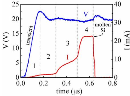
FIG. 2. (Color online) A *p*-type wire with  $L=5.5 \mu\text{m}$ ,  $W\sim 200 \text{ nm}$ , and thickness  $\sim 120 \text{ nm}$  is electrically stressed by a constant voltage pulse.
