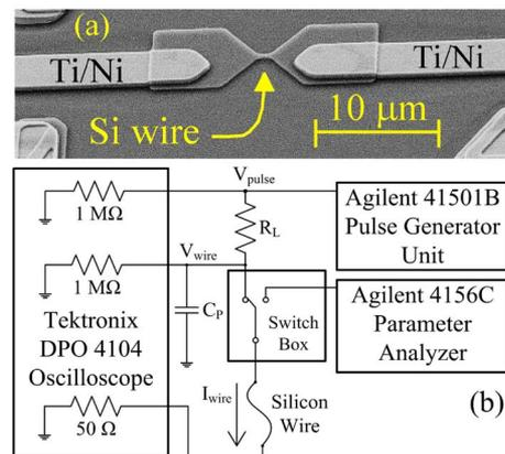
FIG. 1. (Color online) (a) SEM image of a silicon wire with metal contacts and (b) the circuit diagram of the setup used in this experiment. The parasitic capacitances of the load resistor, oscilloscope inputs, and coaxial cables are modeled by the lump capacitor ( $C_P$ ).
