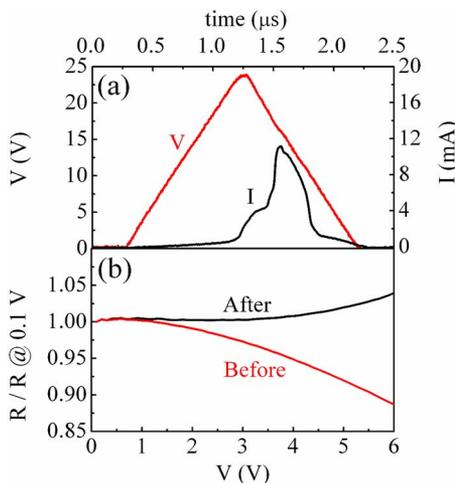
FIG. 3. (Color online) Critical annealing of an *n*-type wire with  $L = 3.5 \mu\text{m}$ ,  $W\sim 130 \text{ nm}$ , thickness  $\sim 80 \text{ nm}$ . (a)  $I_{\text{wire}}$  and  $V_{\text{pulse}}$  vs time during a 24 V triangular pulse. (b)  $R$  scaled by  $R$  at 0.1 V as a function of voltage for dc sweeps taken before and after the pulse. Resistance at 0.1 V is 51.4 k $\Omega$  with negative TCR before the pulse and 4.74 k $\Omega$  with positive TCR after the pulse.
