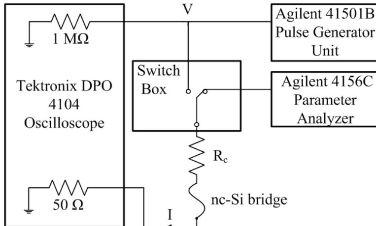
**Figure 1.** Circuit schematic of the experimental setup, where  $R_c$  is the contact-pad resistance. I-V characteristics of the bridges are measured by the parameter analyzer before and after the electrical stress. Switch box switches to pulse generator unit to apply the voltage pulse. Applied voltage pulse amplitude and current through the bridge are acquired by the oscilloscope.
