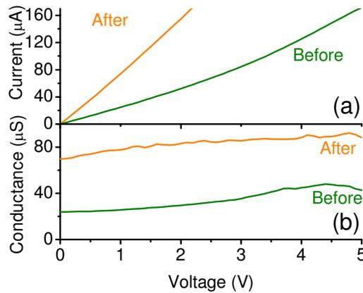
**Figure 4.** (a) I-V characteristics of the bridge shown in Figure 2b, before and after the electrical stress. (b) Conductance of the bridge extracted from the I-V characteristics.
