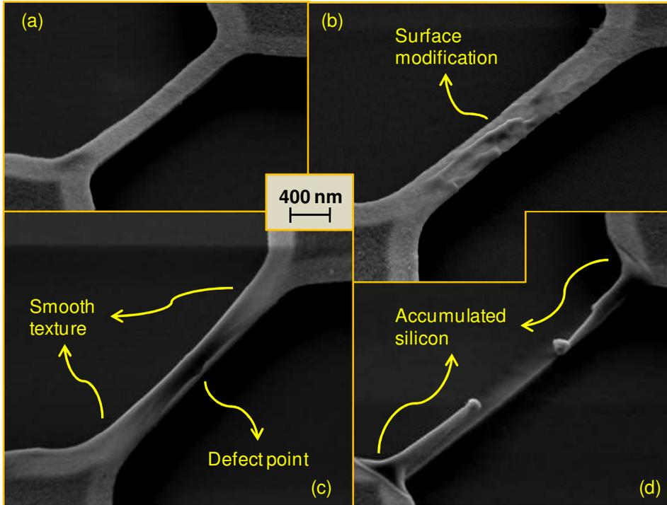
**Figure 2.** (a) An as fabricated 3.5  $\mu\text{m}$  long nc-Si bridge. The bridge and contact pads have uniform nc-Si texture. (b) A 5  $\mu\text{m}$  long bridge stressed with 30 V, 1  $\mu\text{s}$  pulse. Applied electrical stress melted and modified the surface. (c) A 4  $\mu\text{m}$  long bridge stressed with a 25 V, 1  $\mu\text{s}$  pulse. (d) A 5  $\mu\text{m}$  long bridge stressed with 30 V, 1  $\mu\text{s}$  pulse. The bridge is fully molten and broken.
