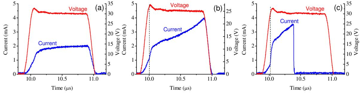
**Figure 3.** V-t and I-t graphs of the bridges (a) in Figure 2b, (b) in Figure 2c, (c) Figure 2d. Vertical dashed lines in (b) and (c) indicate the time when the current drastically increases.
