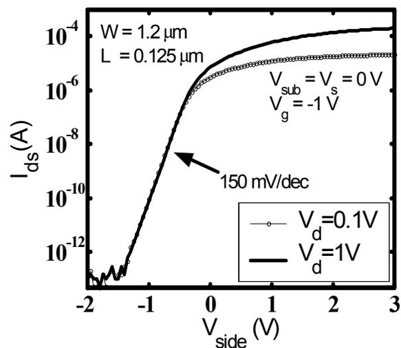
**Figure 5. Drain to source leakage current as a function of  $V_{\text{side}}$ .**
