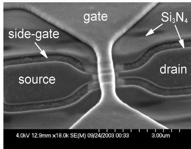
**Figure 3. SEM image before passivation.**
