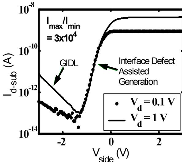
**Figure 4. Reverse-bias leakage current of a drain to substrate diode as a function of  $V_{\text{side}}$ . Area  $\sim 6 \mu\text{m}^2$ , perimeter  $\sim 18 \mu\text{m}$ .**
