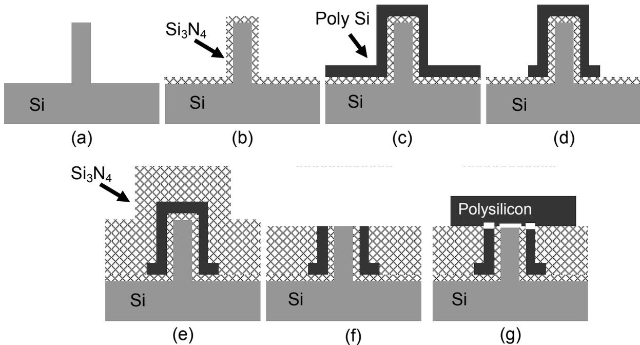
**Figure 2. Composite STI fabrication steps**
