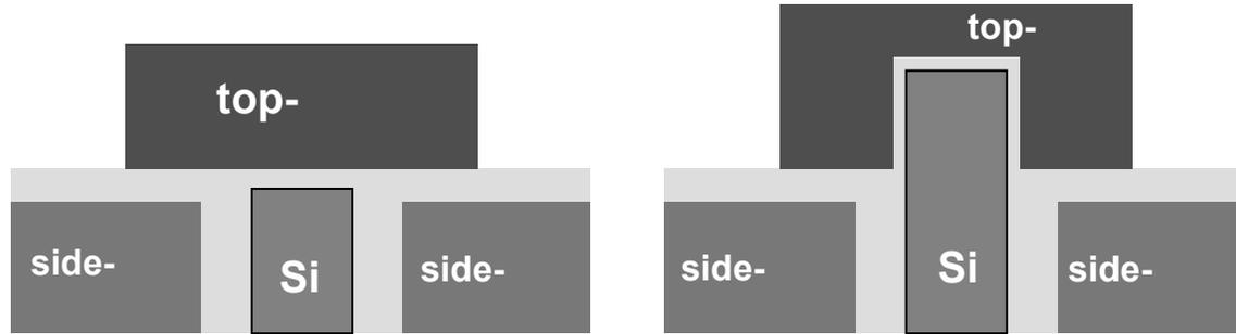
**Figure 6. Planar (left) and tri-gate (right) bulk side-gated device geometries.**
