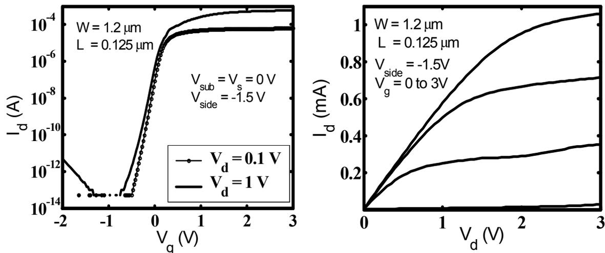
**Figure 7. Drain current as a function of  $V_{\text{g}}$  (left) and drain current as a function of  $V_{\text{d}}$  (right) characteristics for a side-gated bulk tri-gate structure.**
