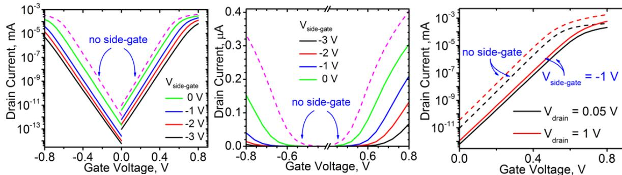
**Figure 4.** Transfer characteristics in log (left) and in linear scale (middle) for an nFET and a pFET with wide-center LER of 3 nm amplitude. Dashed lines are for control devices with no side-gate. Drain bias is 50 mV. High and low drain bias transfer curves (right) for the nFET device with no side-gate and side-gate bias of -1 V, showing reduced DIBL.
