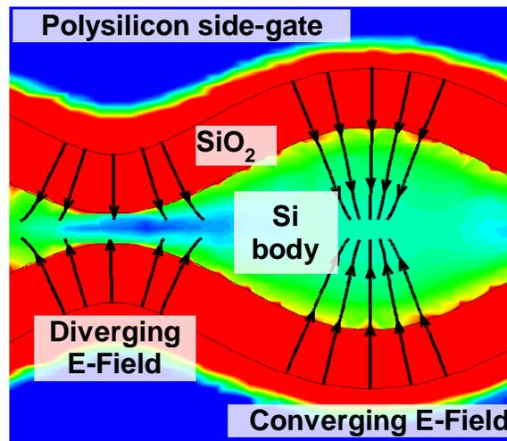
**Figure 2.** Cross-section of a simulated silicon body surrounded by a polysilicon side-gate. Diverging and converging electric fields (arrows) follow LER and electric field intensity (color) is higher on wider regions of the body.
