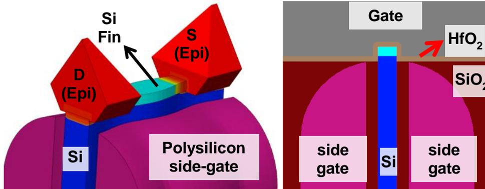
**Figure 3.** Si body with imposed sinusoidal LER of 1 nm amplitude. Gate and dielectrics are not shown (left). Vertical cross-section image at the FET channel center for a side-gated device. Top 3nm (cyan) is covered by the gate (right).
