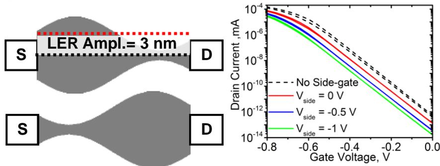
**Figure 5.** Transfer characteristics for a ‘narrow source’ and ‘narrow drain’ pFET cases with no side-gate, and with side gate bias of 0, -0.5 and -1 V. With the side-gate bias, the ‘narrow source’ and ‘narrow drain’ characteristics overlap showing effective reduction of the LER induced variability.
