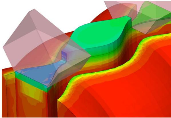
**Figure 1.** 3D electron density graph of a pFET with applied side-gate bias. Red indicates a density of  $1.1 \times 10^{21} \text{ cm}^{-3}$ .
